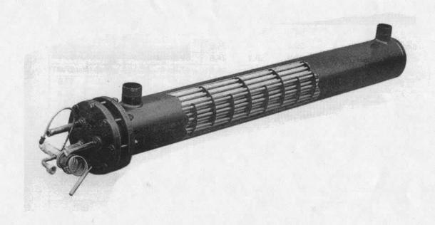
D-X chillers: Capacity ranges 5-300 kW. Dual refrigeration circuits from 200 kW capacity. Superior quality chillers with sand blasted and galvanised shell, copper, stainless steel or titanium tubes. Fitted with cast iron heads.
